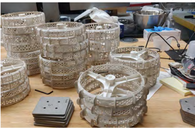
3D-printed CubeRover wheel prototypes.
