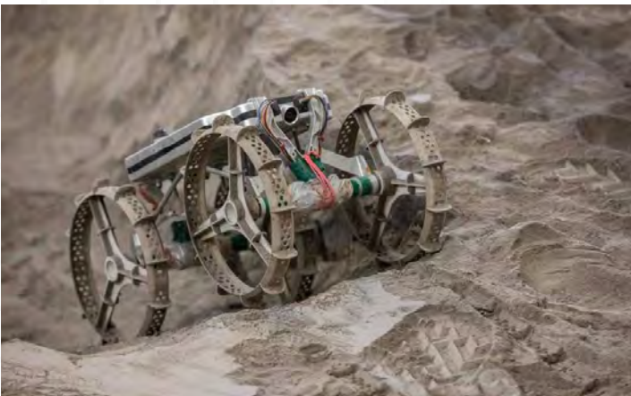
CubeRover mobility testing in regolith simulant.
