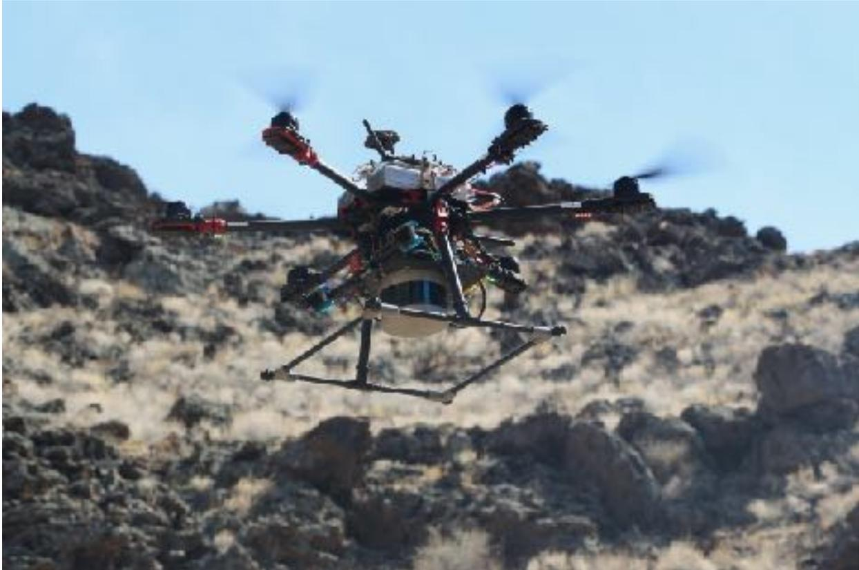
**Astrobotic field-tested their autonomous navigation in Aden Crater in the Potrillo Lava Fields, New Mexico. The geologic features in the field are an analog environment for the Moon or Mars. The team deployed with the SSERVI RIS4E team in March 2018.**
